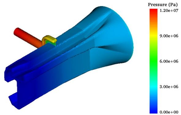
Fig. 16 Pressure distribution in the profile die with polystyrene in substrate and ABS in the cap layer.
