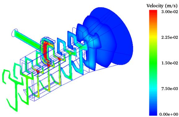
Fig. 13 Velocity distribution in the profile die with polystyrene in substrate and ABS in cap layer.
