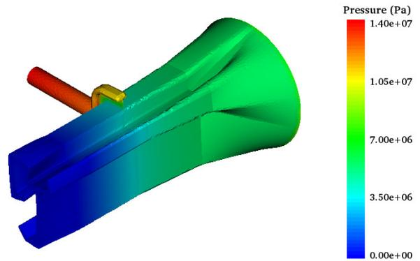
Fig. 6 Pressure distribution in the profile die with ABS in the substrate as well as the cap layer.
