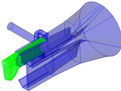
Fig. 10 Interface between the cap layer and substrate with ABS in substrate and polystyrene in cap layer.
