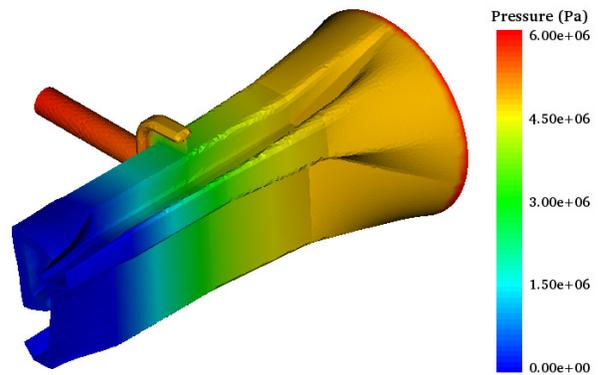
Fig. 11 Pressure distribution in the profile die with ABS in substrate and polystyrene in the cap layer.
