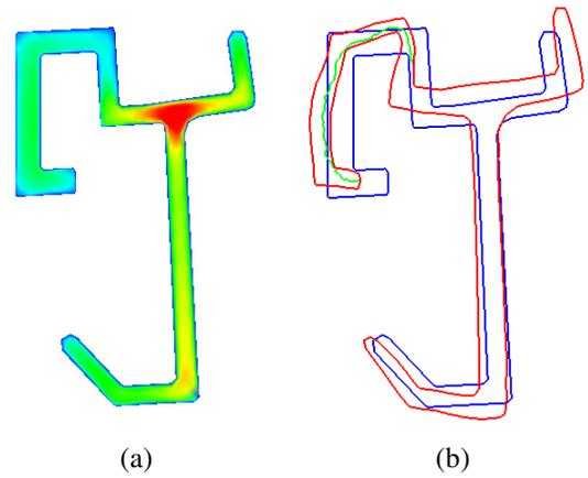
Fig. 14 (a) Velocity distribution at die exit, (b) extrudate profile (red), and interface (green) at the end of the extrudate with polystyrene in substrate and ABS in cap layer. Blue line shows the shape of the profile at die exit.
