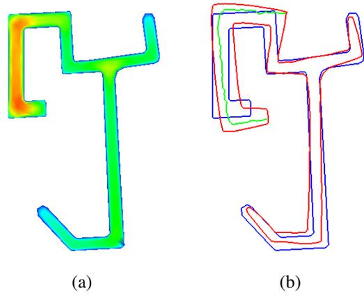
Fig. 4 (a) Velocity distribution at die exit, (b) extrudate profile (red), and interface (green) at the end of the extrudate with ABS in the substrate as well as the cap layer. Blue line shows the shape of the profile at die exit.
