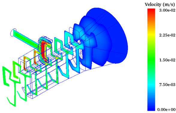
Fig. 3 Velocity distribution in the profile die with ABS in the substrate as well as the cap layer.
