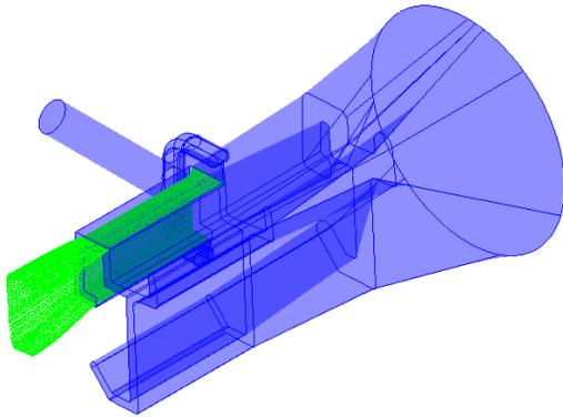
Fig. 5 Interface between the cap layer and substrate with ABS in the substrate as well as the cap layer.
