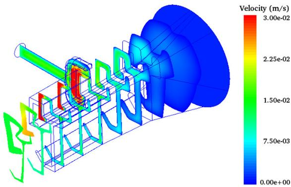
Fig. 8 Velocity distribution in the profile die with ABS in substrate and polystyrene in cap layer.
