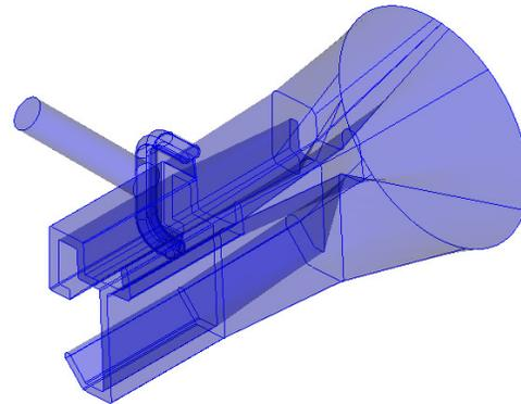
Fig. 2 Geometry of a bi-layer profile die.
