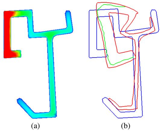
Fig. 9 (a) Velocity distribution at die exit, (b) extrudate profile (red), and interface (green) at the end of the extrudate with ABS in substrate and polystyrene in cap layer. Blue line shows the shape of the profile at die exit.
