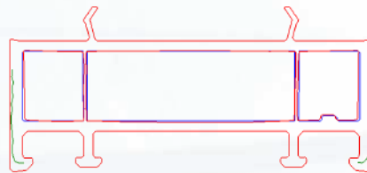
Fig. 5. Predicted shape of the extrudate profile (red), layer structure (green), and shape of the profile at the die exit (blue).
